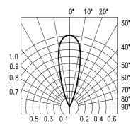
Fig.5 Luminous Intensity vs.
